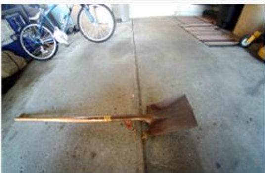
OmniVision Approach Optical distortion with lens only distortion correction
